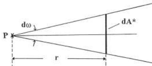
Fig. 2. Schematic determination of the photometric law of distance.
