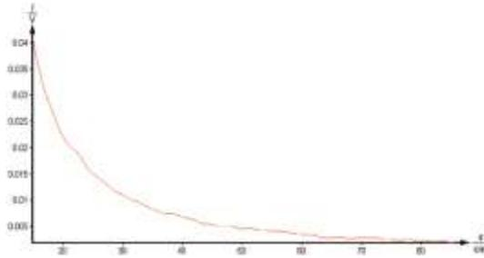
Fig. 3. Luminous intensity as a function of distance (Lamp – Photocell)
